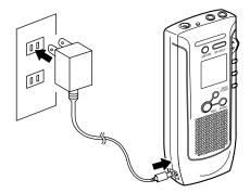
Plug the optional AC adapter into a household power outlet and connect the power plug to the recorder's power connector (DC 3 V) as shown in the illustration. Do not connect the AC adapter to the recorder during recording. Always stop recording before connection. Otherwise it may not be possible to play back the voice data being recorded.
